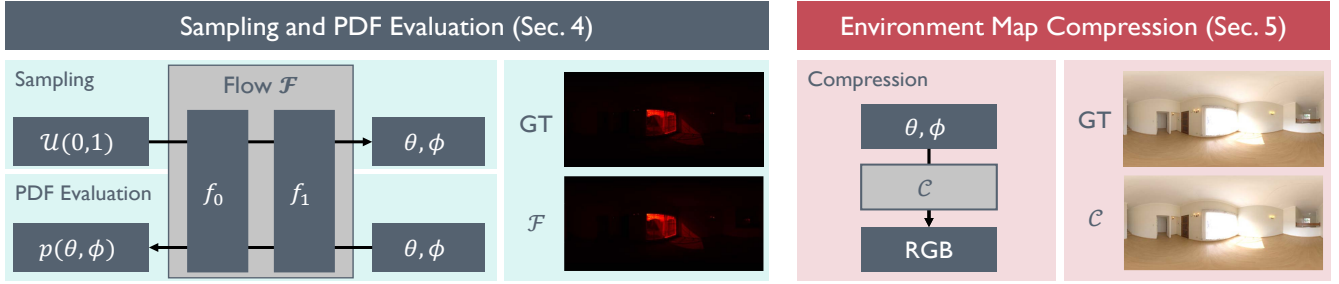
Figure 2: Overview of NEnv. We propose an invertible generative neural network \mathcal{F} (i.e. a normalizing flow) which simultaneously learns to sample directions (\theta, \phi) from an environment map, as well as evaluating the probability of a given direction. This model, illustrated on the left, can be integrated seamlessly into path tracer render engines, allowing for efficient multiple importance sampling. We additionally use an implicit neural representation \mathcal{C} (second column) which learns to map from directions to linear RGB values, allowing for faster evaluation.
