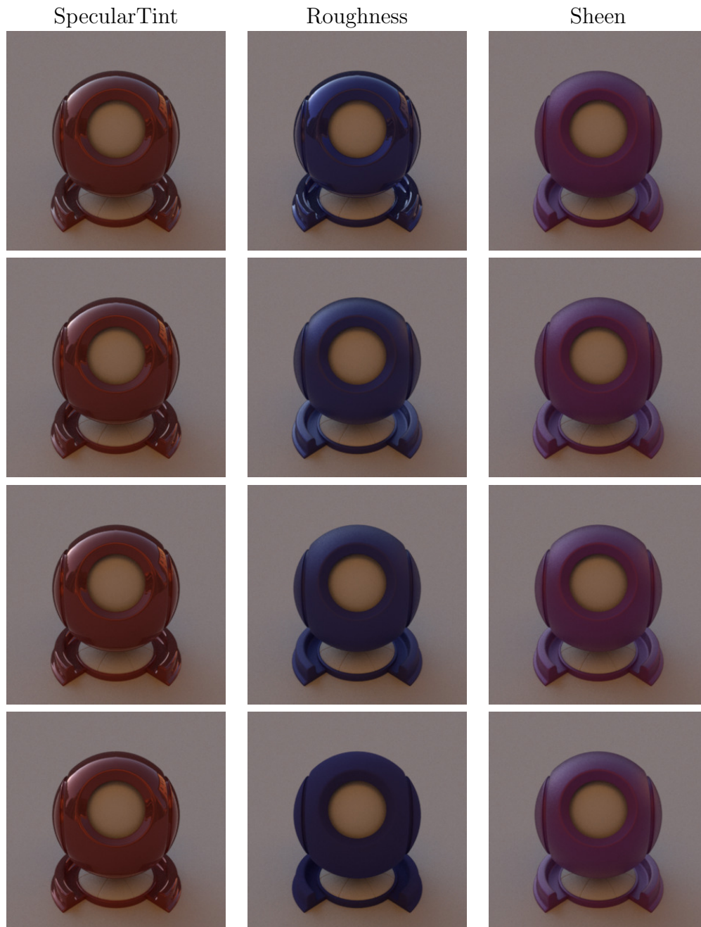
Figure 7.2: Rendered examples of the Disney Principled BRDF varying its SpecularTint , Roughness and Sheen parameters
