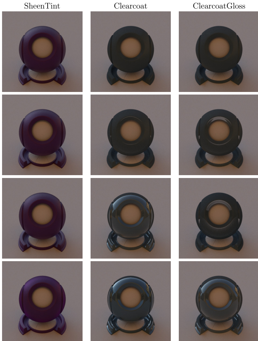
Figure 7.3: Rendered examples of the Disney Principled BRDF varying its SheenTint , Clearcoat and ClearcoatGloss parameters
